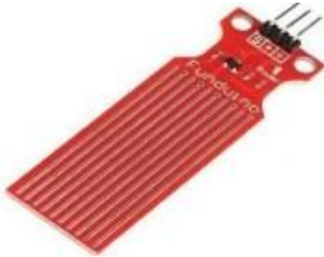
Fig 6. Water Level Sensor
